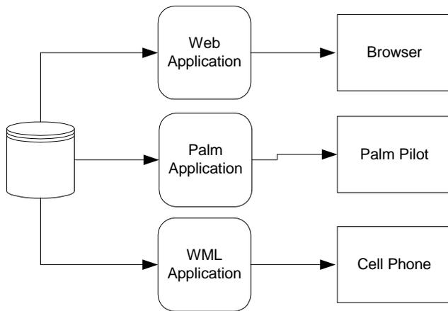
We have a serial path from each device back to the database. Adding a new device means adding a new application that produces the output required for that device.
