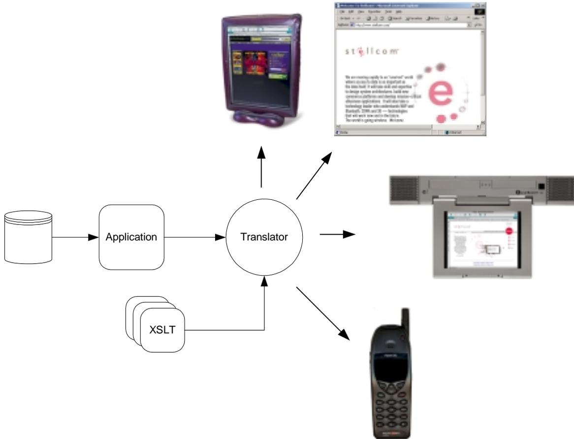
In this case, only one application exists. It runs against the back-end database, and produces an XML stream. A "translator" takes this XML stream, and applies an XSLT transformation to it. Every device could either use a generic XSLT, or have a specialized XSLT that would produce the required device-specific output. The transformation occurs on the server, meaning that no special client capabilities are required.
